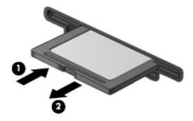
**NOTE:** If the card does not eject, pull the card out of the slot.
